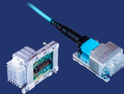
10X10 Gbps Parallel Optic Transmitter or Receiver 120 Gbps
