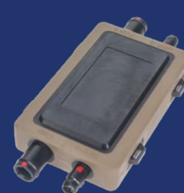
STAR-PAN NG 1/2 P/N TS2-011 Our smallest hub with one EUD port, one pan port and two universal power ports
