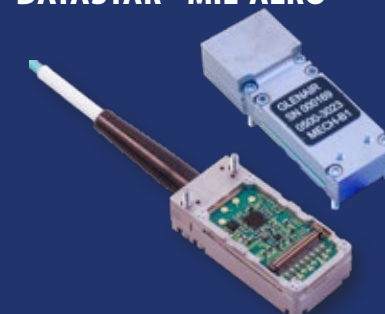
Low-Profile Quad Parallel Optical Transceiver 28 Gbps
